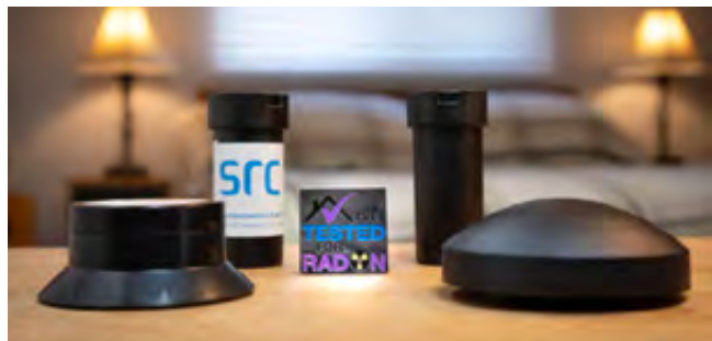
Examples of alpha-track radon detectors (passive detectors). Photo courtesy by Take Action on Radon.
